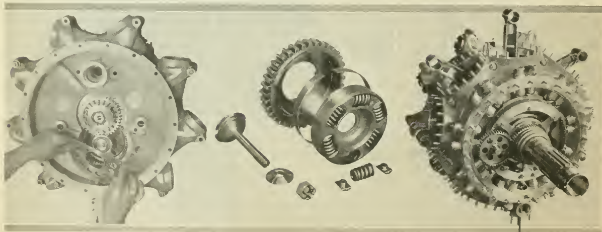
Pratt & Whitney S1H1-G engine impeller and supercharger drive, spring coupling (clutch) and power section of direct drive engine
